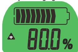
4. When the charge or discharge current is less than backlight off current, coulometer enter a low power state and backlight off. And TR16 can memory the capacity.
