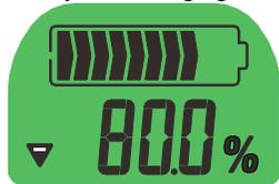
3. Break the load , and connect the charger. When the charge current is higher than backlight on current , backlight blinking (if backlight on , the RS+ and RS- are inversely), and display charge indicator ,indicate battery is charging.
